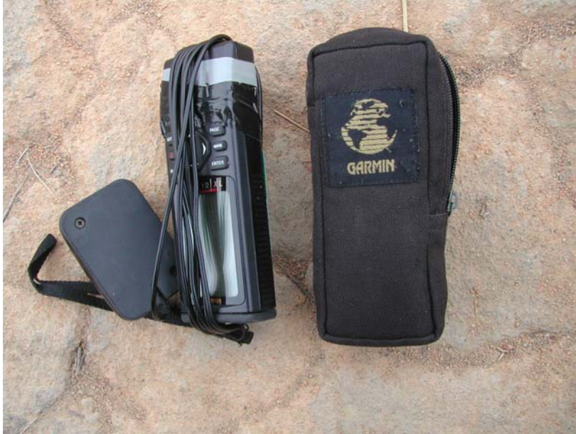
Fig. 9. Correct storage of antenna and GPS unit.
